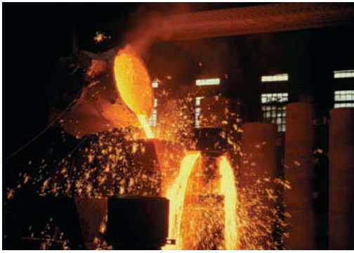
Monitoring temperature of molten metal prior to and during pouring ensures correct metallurgical properties.
