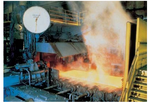
Accurately measuring temperature of slabs, billets, or blooms on a hot rolling mill ensures product uniformity.
