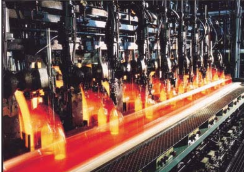
From the molten state through to the cooling process, continuous temperature monitoring ensures that glass retains its properties as it travels through the manufacturing process.
